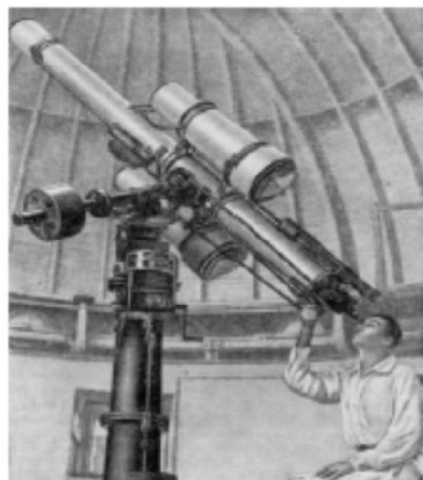
Double astrograph with 120 mm Unar lenses
